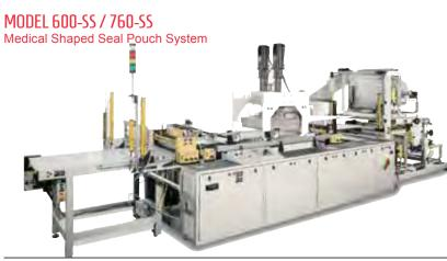
The Shaped Seal Pouch System converts peel-able chevron shaped surgical pouches at speeds up to 220 cpm. Products include shaped seal pouches, surgical peel pouches, self-seal surgical peel pouches and autoclavable tube stock made from paper or Tyvek® sealed to PET/LDPE or PET/PP.
