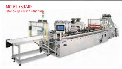
Servo-actuated sealing technology replaces costly, maintenanceintensive air cylinders, while providing a stable and consistent process at speeds up to 220 cycles per minute.
