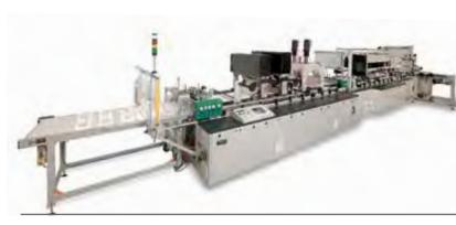
In chevron (shaped) peel pouch configuration, the 760-SSHB combines two webs of material, making pouches in single or multiple lanes across the width of the machine. In medical header bag configuration, the machine will process two main webs of poly material and one web of Tyvek®, for high-quality header bags in a variety of sizes.
