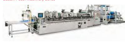
Produces side-sealed and side-gusseted bags of exceptional quality at high-performance production speeds of up to 100 cycles per minute. Equipped with the latest in CMD process-driven innovation and convenient operational features. Other customized configurations are available.
