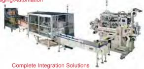
Model 0330HSW Global High-Speed Overlap Bag Winder shown with integrated pick-and-place robotics and conveyor system, case erector and closer.
