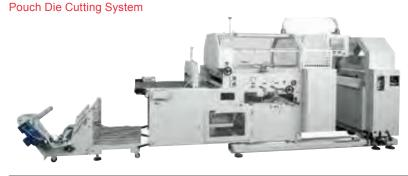
This free-standing, intermittent-motion die cutter can be easily integrated with existing pouch converting equipment. It is capable of deliverying up to 4 lanes of flat or bottom-gusseted pouches. The large, servo-actuated cutting platen has enhanced cutting force for repeatable die cutting of large, heavy gauge or intricately shaped pouches.
