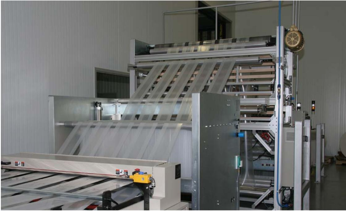
*ABOVE: Polykar's new CMD 1400DBS Bottomseal System converts up to 8 lanes of film, producing up to 1,000 bags per minute.*
