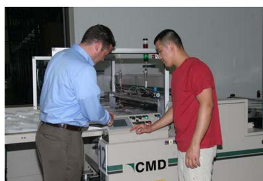
Along with the multiple-lane capability, the system handles film gauges from .25 mil star-seal folded material to 8 mil non-gusseted tubing sheeting; gusseted or non-gusseted bags. The line runs bulk packaging products: bread bags, freezer bags, pound bags, trash bags and general use bags.
