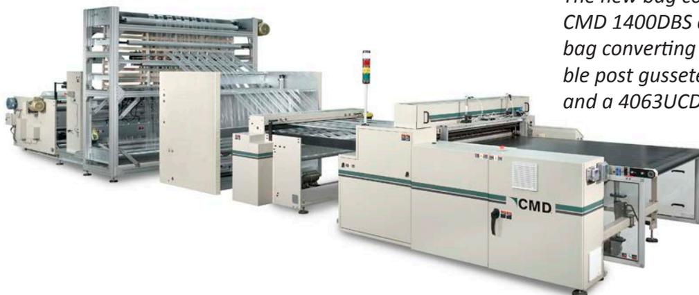
The new bag converting line includes the CMD 1400DBS clamp-stacking, bottomseal bag converting system with a 7208BPG bubble post gusseter, 7207BSS bubble slit sealer and a 4063UCD parent-roll unwind.
