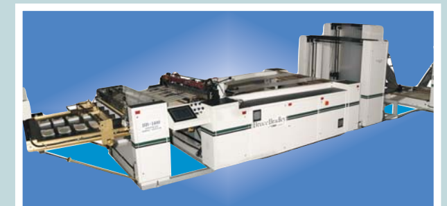
Side Weld Bag Machines: (2) 56 in solid machines, each with unwind 56 in split-lane with two unwinds
